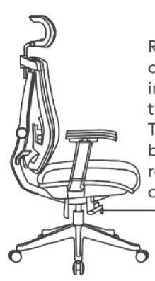
Rotate the handle clockwise to increase the back tilt tension.
